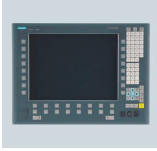
The SINUMERIK TP 015AT operator panel front with 15" TFT color display,  $1024 \times 768$  pixels (XGA) and touch screen supports the distributed installation of the operator panel front and control. The SINUMERIK TP 015AT operator panel front contains a membrane keyboard with 62 keys as well as  $2 \times (8+2)$  horizontal and  $2 \times 8$  vertical softkeys and an integral mouse.
