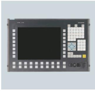
The SINUMERIK OP 012 operator panel front with 12.1" TFT color display with a resolution of  $800 \times 600$  pixels (SVGA) features a 59-key membrane keypad as well as  $2 \times (8 + 2)$  horizontal and  $2 \times 8$  vertical softkeys. The integral mouse provides an additional method of machine control. The  $2 \times 8$  vertical softkeys can be used as direct keys in the PLC.
