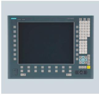
The SINUMERIK TP 015A operator panel front with 15" TFT color display with a resolution of  $1024\times768$  pixels (XGA) and touch screen features a 62-key membrane keyboard as well as  $2\times(8+2)$  horizontal and  $2\times8$  vertical softkeys and an integral mouse. The  $2\times8$  vertical softkeys can be used as direct keys in the PLC.
