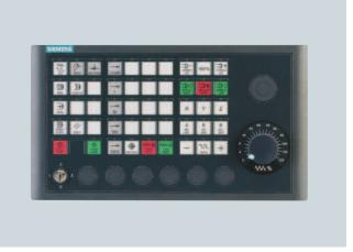
The SINUMERIK MCP 310 PN machine control panel with membrane keys is designed to permit user-friendly, well-structured operation of the machine functions. It is suitable for machine-level operation of milling, turning, grinding and special machines.
