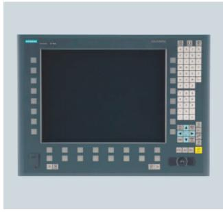
The SINUMERIK OP 015A operator panel front with 15" TFT color display with a resolution of  $1024\times768$  pixels (XGA) features a 62-key membrane keyboard with 2  $\times$  (8 + 2) horizontal and 2  $\times$  8 vertical softkeys and an integral mouse. The 2  $\times$  8 vertical softkeys can be used as direct keys in the PLC.
