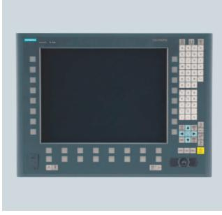
The SINUMERIK OP 015AT operator panel front with 15" TFT color display, 1024  $\times$  768 pixels (XGA), supports the distributed installation of the operator panel front and control. The SINUMERIK OP 015AT operator panel front contains a membrane keyboard with 62 keys as well as 2  $\times$  (8 + 2) horizontal and 2  $\times$  8 vertical softkeys and an integral mouse.
